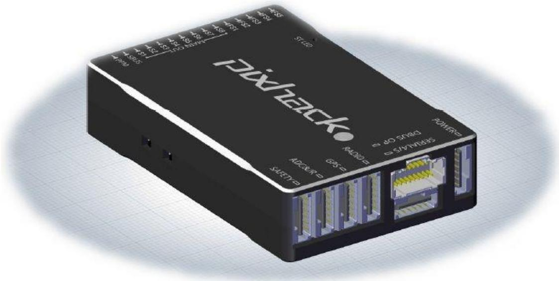
Pixhack is a flight controller, based on Pixhawk hardware architecture platform, designed and produced by CUAV. As the main architectural hardware the same with pix, so fully compatible with the 3DR APM firmware and pix native firmware.
