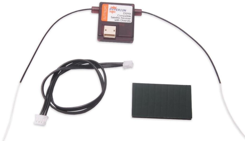
**This DSMX compatible diversity satellite receiver will extend your range and increase your radio link robustness. Just in case the antennae on your main receiver cannot receive a signal due to its orientation or airframe shadow (due to carbon fiber), this satellite will use one of its two antennae to receive your radio signal (diversity), vastly improving the chance that you receive proper commands from the transmitter.**
